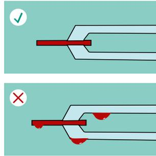
**Note!** Check that the capillary part is completely filled. **Do not wipe the sample collector!** If there is excess sample on the sample collector, discard the sample collector.
