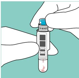
**4** Close the cuvette tightly with the easy CRP reagent cap. Do not press down the turquoise inner part of the reagent cap. Perform the test within 2 hours.
