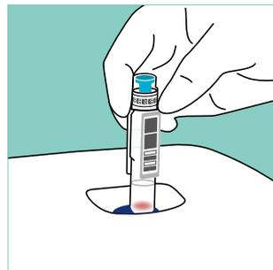
**5** Choose **Measure** on the display of the QuikRead go instrument. Insert the cuvette into the measurement well of the instrument. The barcode should be facing you.
